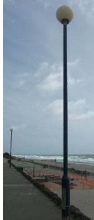
Steel light poles with single bud lights. These light poles have been painted.
