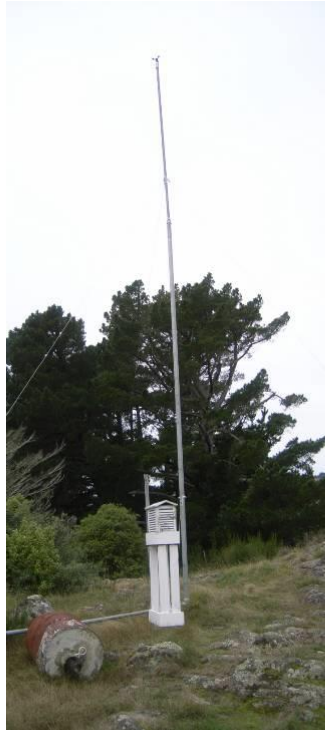
Fire information weather station. The white box is a Stevenson screen and contains sensors. The tall pole is an anemometer pole with an anemometer on top.
